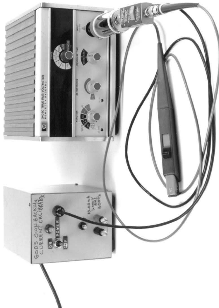
Figure C9a • Complete Current Probe Test Set Includes Probe, Amplifier, Calibrator and Thermally Based RMS Voltmeter. Accuracy Is 1% to 10MHz
