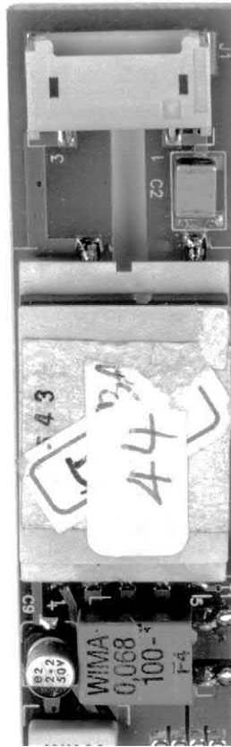
Figure G5 • Transformer Output Terminals, Ballast Capacitor and Connector Are Isolated at End of Board. Slit Prevents Leakage
