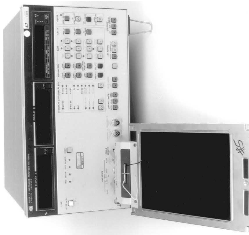
Figure 8.13 • Measuring Lamp Wire to Display Frame Capacitance. Technique Gives Lead Wire-to-Frame Loss Information but Not Lamp-to-Foil-or-Frame Loss Data. Lamp Must Be Energized Before Its Parasitics are Measurable
