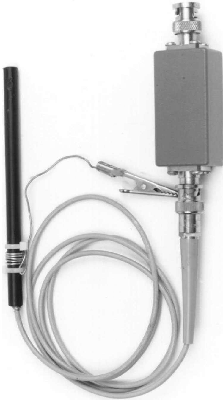
Figure C15 • The Trigger Probe and Termination Box. Clip Lead Facilitates Mounting Probe, Is Electrically Neutral
