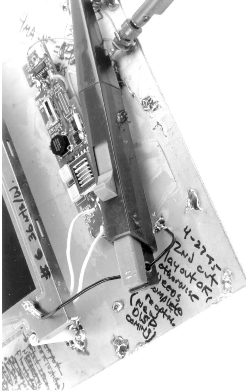
Figure C9b • Current Probe Measuring Display Frame Parasitic Current. “Clip-On” Capability Allows Measurement at Any Point in Lamp Circuit
