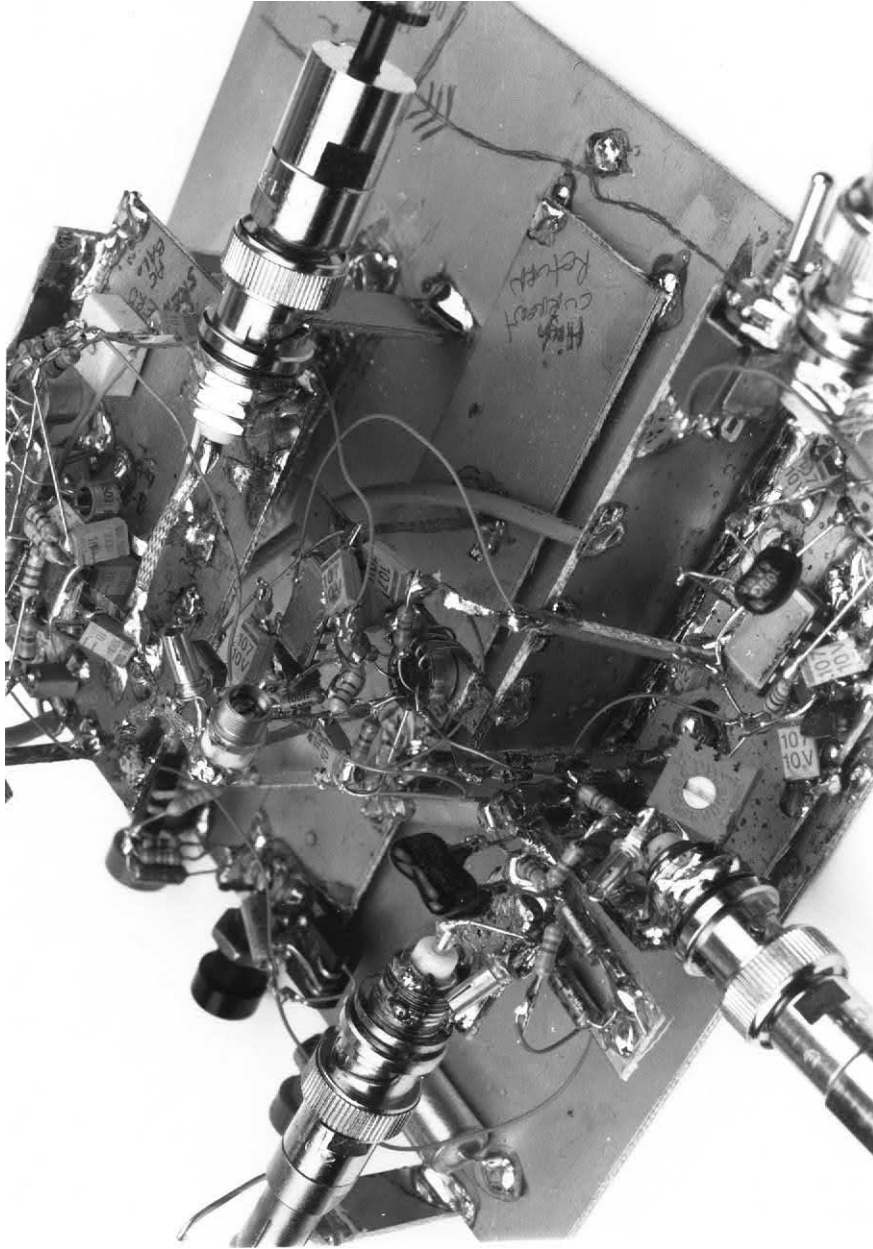
Figure E5 • Input Bridge and Amplifier-Under-Test (AUT) Detail. Pulse Generator Enters Lower Left. Input Bridge Is IC Can (Photo Center); AUT Just Above. AUT Feedback Trim Capacitor Is Upper Center. IC Behind Trim Capacitor Is Bridge Driver Amplifier. Sampling Bridge (Partial) Is Photo Upper. Probe (Photo Extreme Right) Monitors Sampler Input. FET Probe (Photo Extreme Left) Measures Delay Compensated Input Pulse
