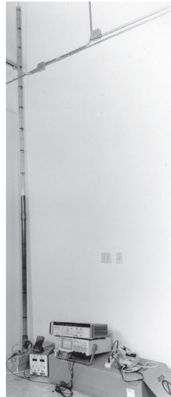
Figure 38.150 • Test Setup for Water-Column Sensor
