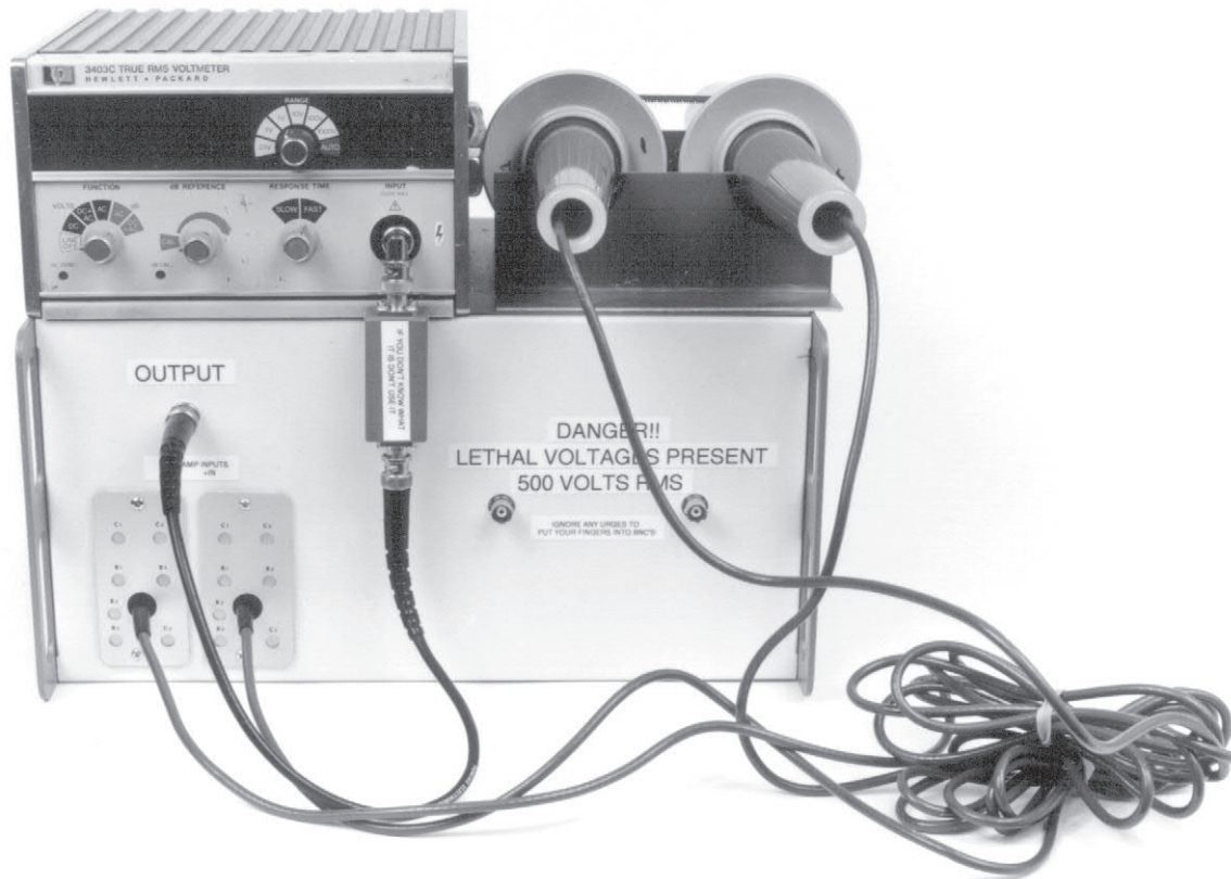
Figure C16 • Complete Differential Probe and Calibrator. BNC Outputs Provide Precision, Floating 500V RMS Calibration Source to Check Probe/Amplifier Section
