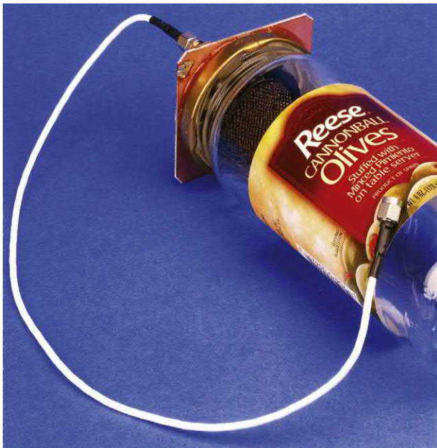
Figure 27.2 • Photograph Details Cap Assembly, Partially Views Glass Enclosed Measurement Path. Ultrasonic Transducer Visible Within Cap. Stiffening Plate, Bonded to Cap Top, Prevents Ambient Pressure or Temperature Changes from Deforming Thin Metal Cap, Promoting Measurement Path Length Stability. Coaxial Header Provides Transducer Connections
